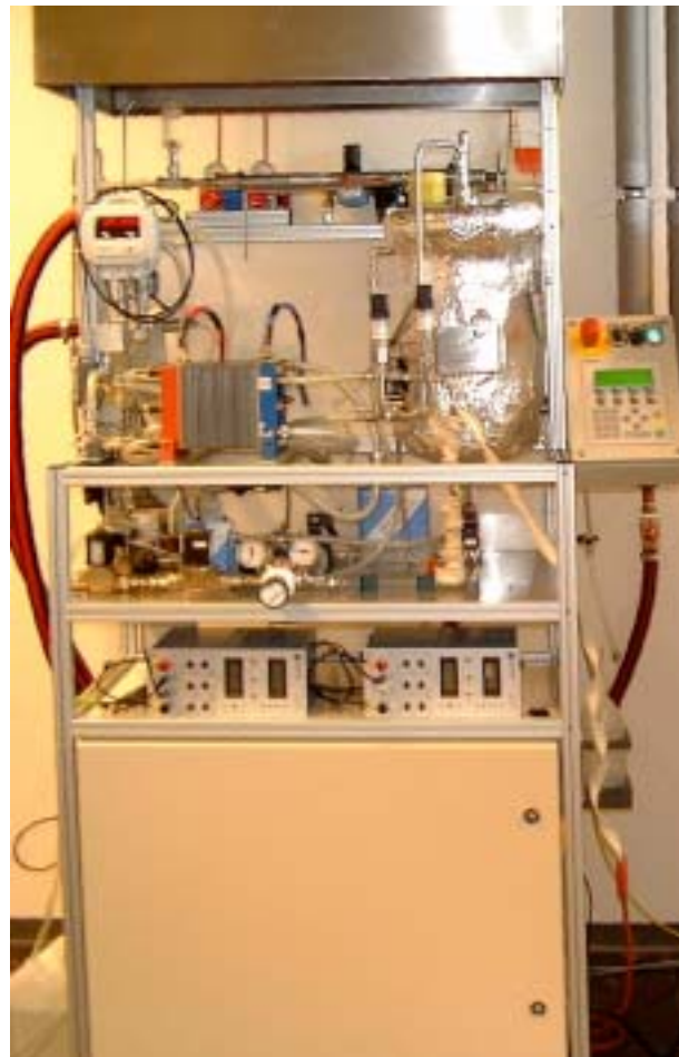
Fig. 3: ZSW PEFC-test bench for educational purposes (1 kW)
